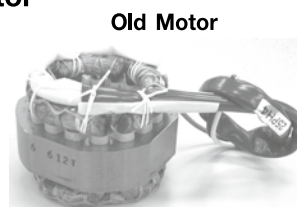
Picture 3 : Old motor is half assembly by manual whereas new motor is proceeded by machine and the cores are independently divided.
